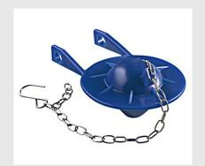
To check for a leaking toilet flapper, add a few drops of food coloring or leak detection tablets to the toilet tank. Wait 10 minutes, then check for colored water in the bowl. If there is any color in the toilet bowl, you have a leaking flapper.
